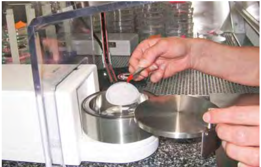
The increase in weight of the particle filter is monitored for emissions measurement.
