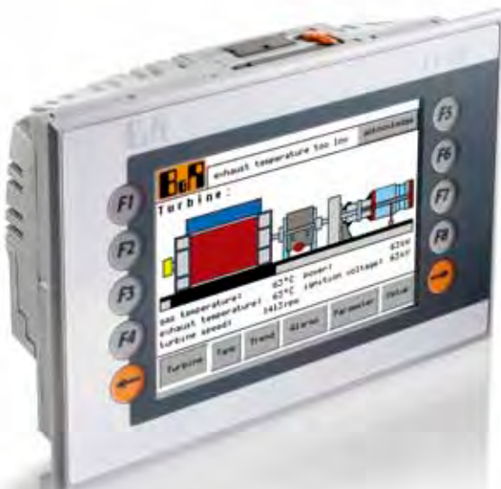
All measurement data is recorded and evaluated using a Power Panel.
